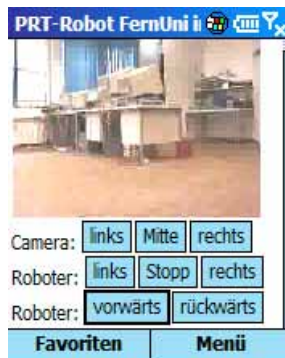
Figure 8: Screenshot of mobile application, video stream and asynchronous Javascript (similar to AJAX) integrated in mobile IE
