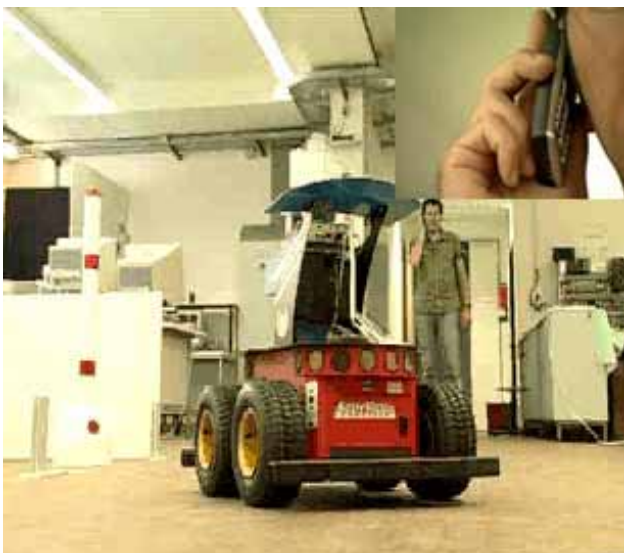
Figure 9: Pioneer 3AT mobile robot controlled by speech via cell phone
