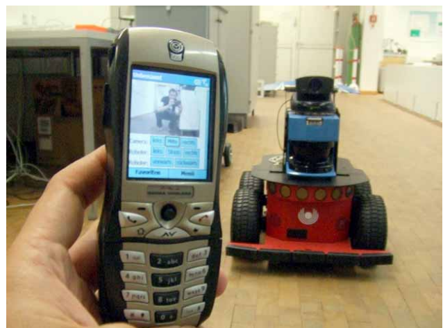
Figure 7: Pioneer 3AT mobile robot controlled by Windows Mobile smartphone
