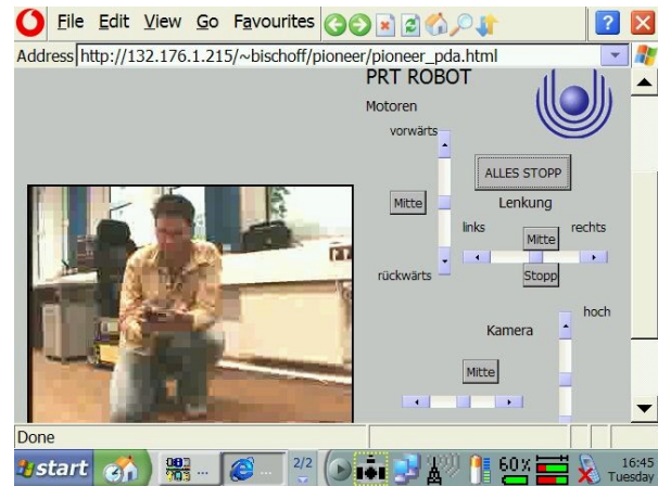
Fig. 3. Web and Java AWT based GUI on a smartphone (640x480 pixel)
