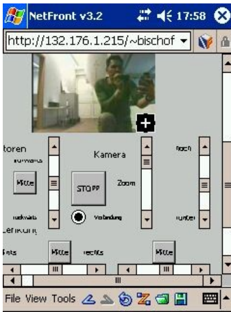
Figure 5: Pioneer robot remote control applet with kuttpech video stream on a PocketPC
