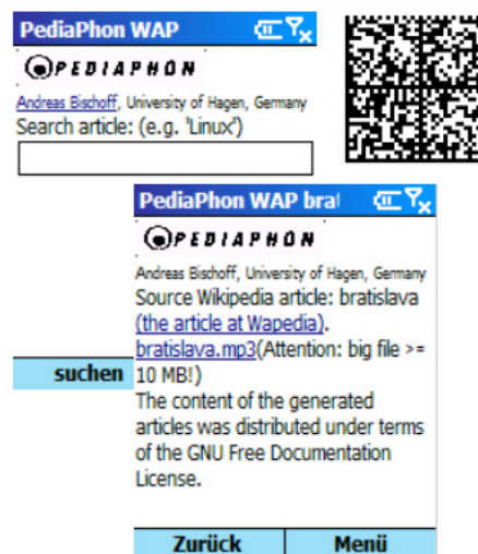
Figure 1: WAP interface of the Pediaphon speech output of Wikipedia articles and 2D barcode representation of the corresponding URL
